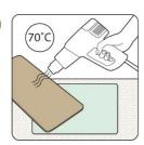
Cover surface with a silicone mat. Heat Thibra with a hot air gun or in an oven, the material will become flexible and soft. Best deformable at 70 °C. Careful: the material is too hot when it becomes shiny.
