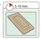
Let Thibra cool down for 5-10 minutes. If multiple layers are used, the cooling period will be longer. If you want to adjust the shape later on, the material can be reheated.
