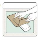
Cover the object with the heated material. Press Thibra evenly onto the surface. You can use your hand or sculpting tools to copy the details of the underlying object.
